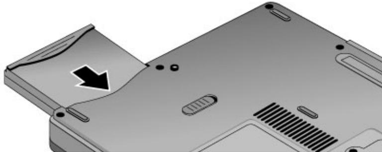
Once you have installed the battery, you can connect the AC adapter to the notebook and charge the battery while you work.
