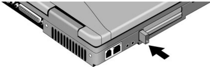
3. Press the eject button again to eject the PC card, and pull the card out of the notebook.
