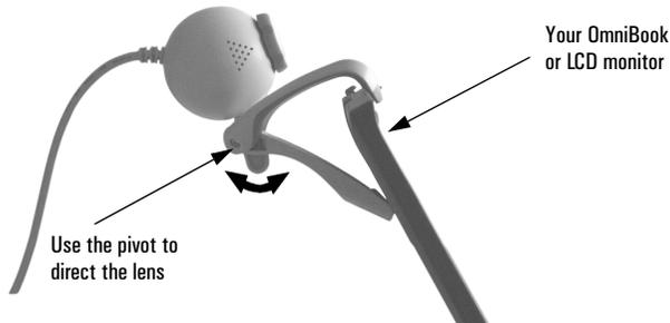
If you are using your USB camera with the camera base, place it on your monitor with the Logitech logo on the camera rest facing you (see picture below). Direct the lens by tilting the camera eye upwards or downwards until the picture in the Logitech QuickCam Test window is satisfactory.
