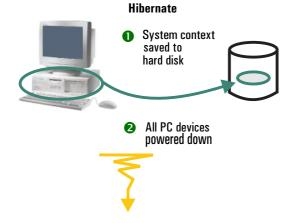
The PC's system context (contents of main memory, position of all programs, etc.) is stored on hard disk and then all devices are powered off. The PC goes into state S4.
