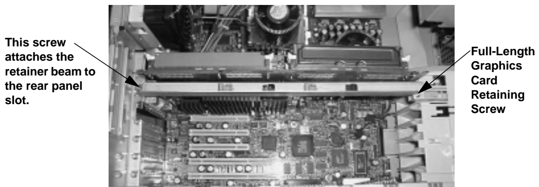
Figure 10-14 Graphics Card Retainer Beam
