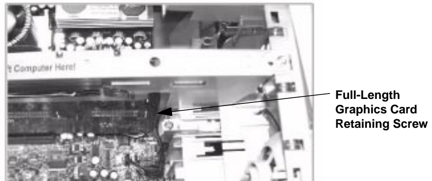
Figure 10-13 Full-Length Graphics Card Retaining Screw
