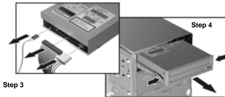
Figure 10-20 Removing the Old Drive
