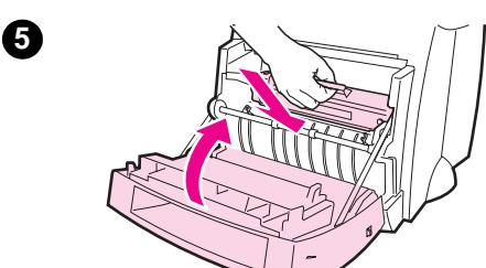
A piece of jammed paper can tear while being removed. Use the following procedure to remove any small pieces of paper left in the printer.
