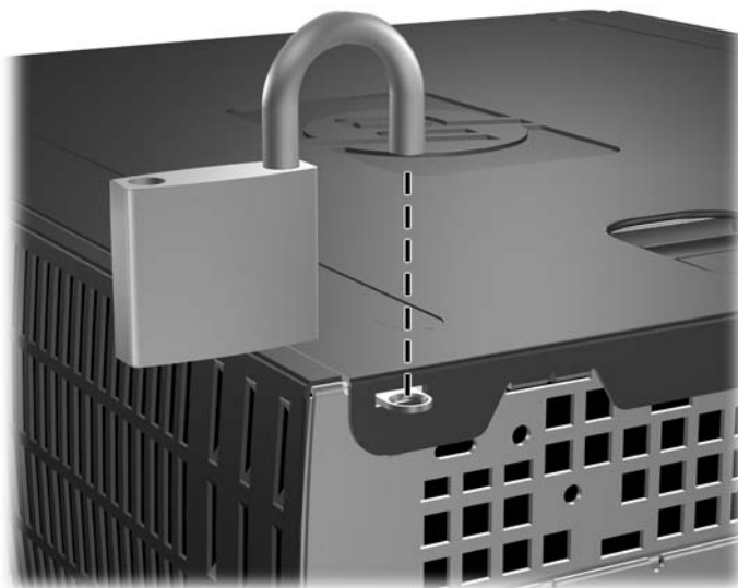
Installing a Padlock
