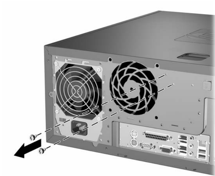
Figure 2-1 Removing the Smart Cover Lock Screws
