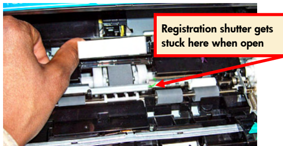
The pick roller assembly has moved to the right
