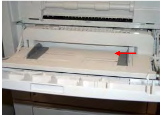
Tray 2 shutter closed (incorrect)
