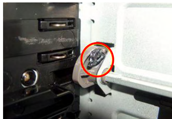
Rotating SCIP cams out of the way
