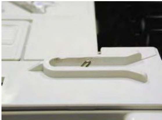
Deformed or bent grounding spring
