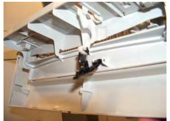
The shutter arm mechanism should move freely
