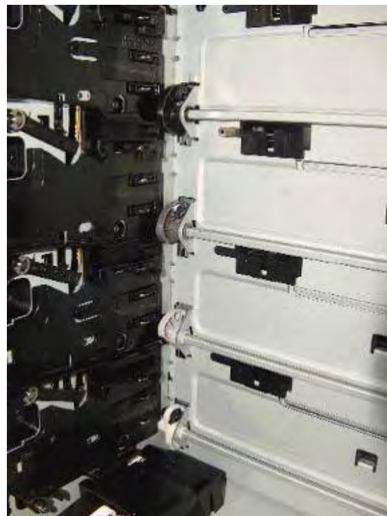
Developer Alienation Cams after successful SCIP cam roll over
