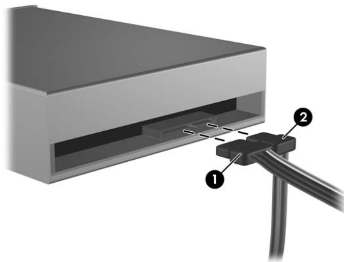
Figure 2-23 Disconnecting the Optical Drive Power and Data Cables
