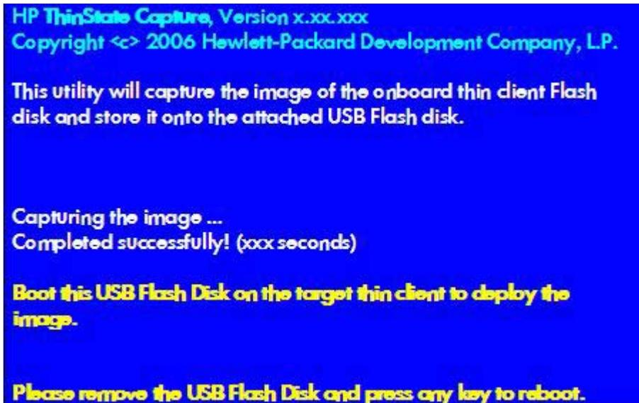
You can now use the USB flash drive to deploy the captured image to another HP thin client of the exact same model and hardware with equal or greater flash size capacity.
