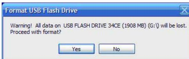
4. Click **Yes**. The HP ThinState Capture tool formats and makes the USB flash drive bootable. HP ThinState Capture will now reboot the system.
