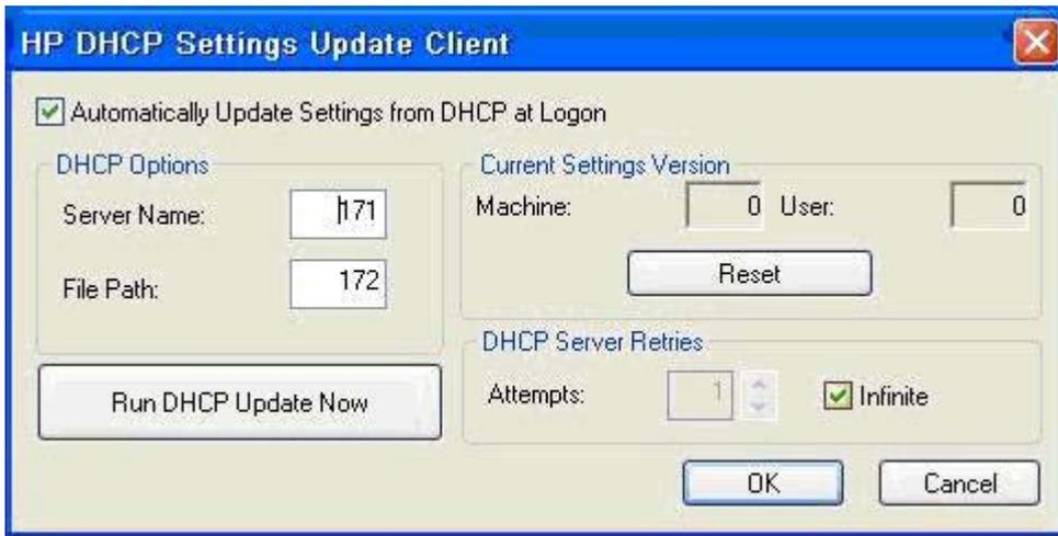
The settings are applied through an .INI file that uses a subset of parameters from Microsoft's sysprep.inf as well as several XPe/HP-specific keys. XPePrep can run by specifying a local .INI file to be processed, or it can be used in conjunction with DHCP and FTP servers to automatically apply settings across multiple clients on a network.
