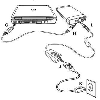
**4** Plug the rectangular end of the USB cable (**G**) into an available USB port on your computer. Plug the square end of the USB cable (**H**) into the USB connector on the back of the drive.
