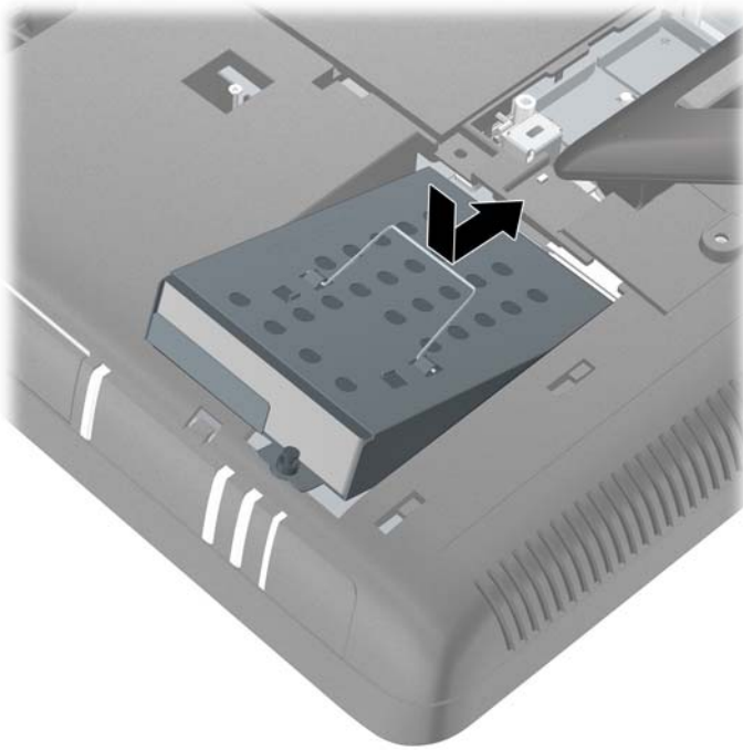
Figure 2-25 Installing the Hard Drive Cage
