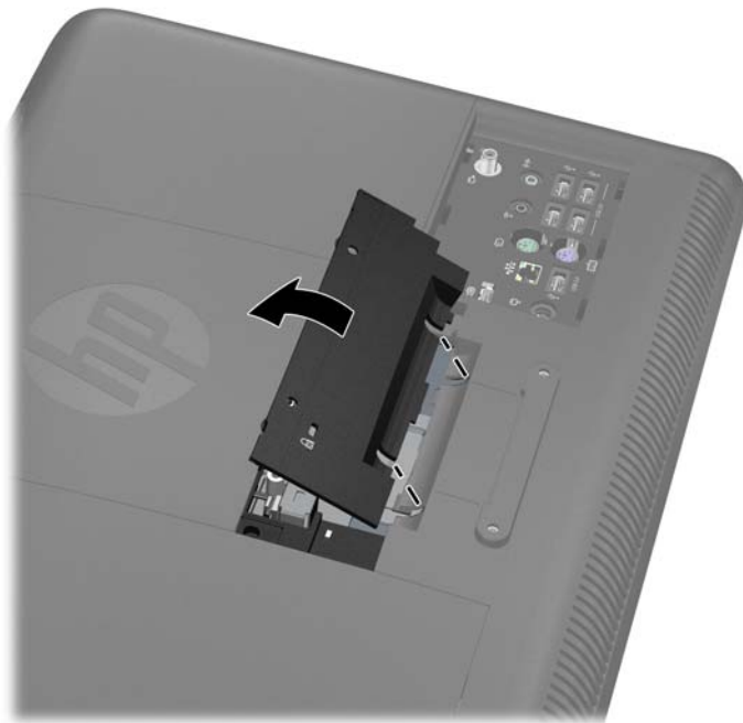
Figure 2-31 Replacing the Center Access Panel
