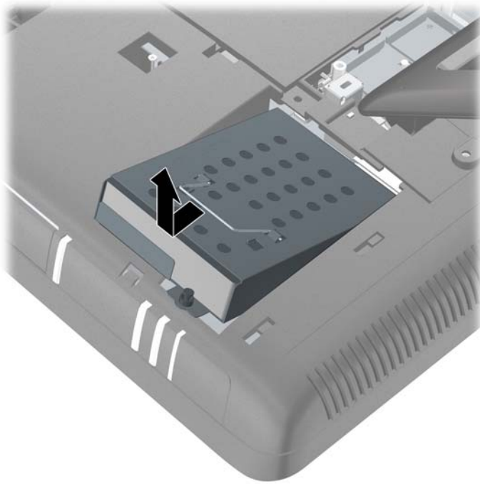
Figure 2-20 Removing the Hard Drive Cage
