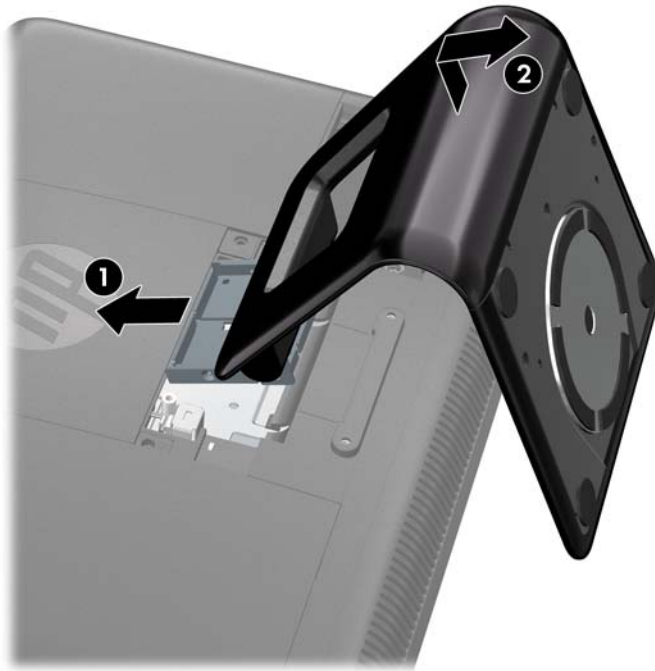
Figure 2-29 Removing the Stand
