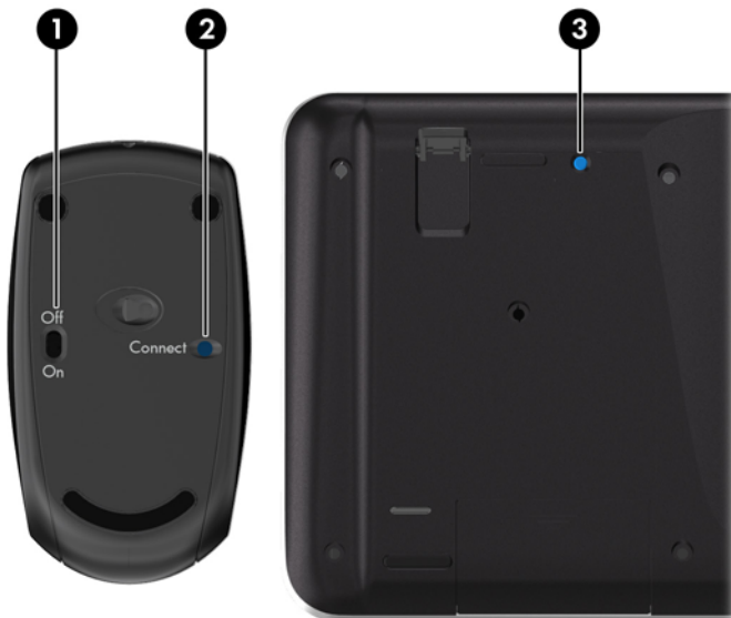
Figure 2-34 Synchronizing the Wireless Keyboard and Mouse
