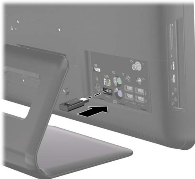
Figure 2-33 Installing the Wireless Receiver
