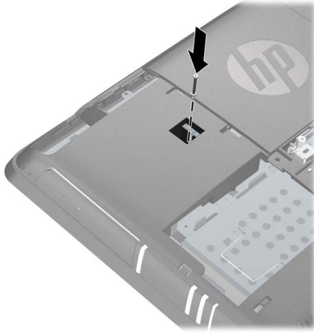
Figure 2-18 Installing the Optical Drive Security Screw
