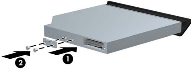
Figure 2-16 Installing the Optical Drive Security Bracket
