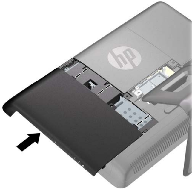
Figure 2-8 Replacing the Drive Access Panel
