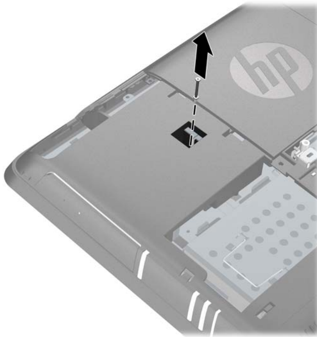
Figure 2-13 Removing the Optical Drive Security Screw
