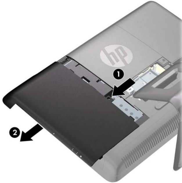
Figure 2-7 Removing the Drive Access Panel
