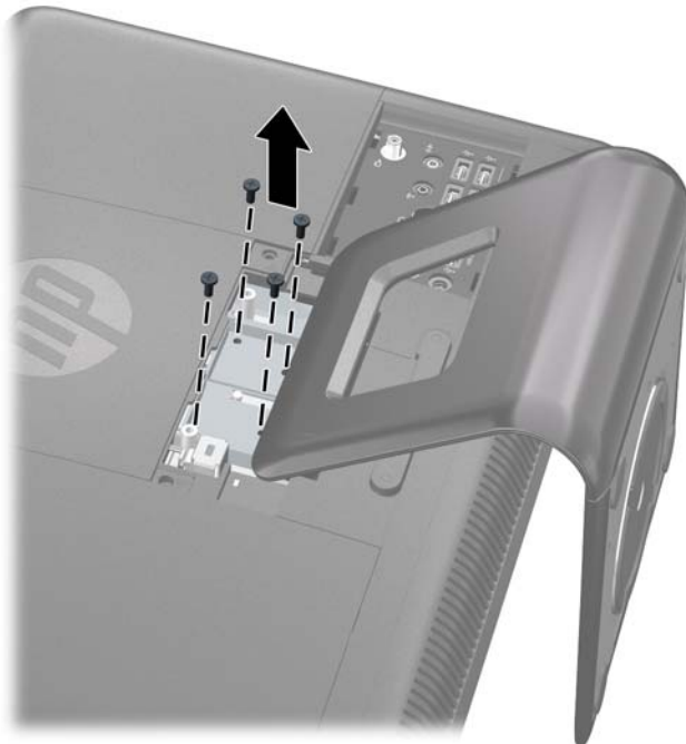
Figure 2-28 Removing the Stand Screws
