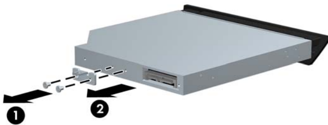
Figure 2-15 Removing the Optical Drive Security Bracket
