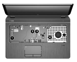
6. Remove the Phillips PM2.5×4.0 screw that secures the top cover to the computer.
