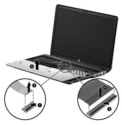
Reverse this procedure to install the keyboard.
