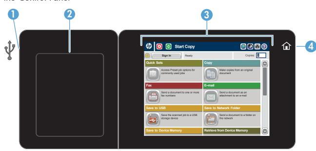
USB port for printing documents directly or saving scanned documents to a USB flash drive Supported file types:
