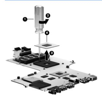
Reverse this procedure to install the processor.
