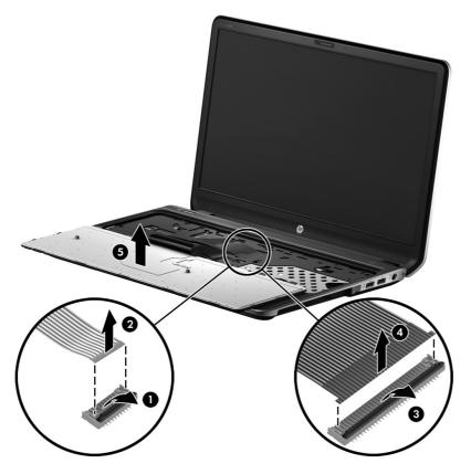
Reverse this procedure to install the keyboard.
