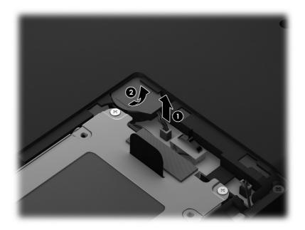
**3.** Remove the RTC battery.
