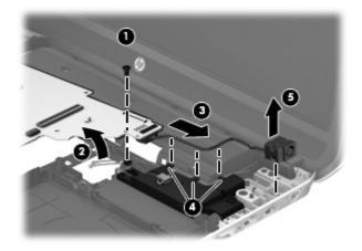
5. Remove the power connector cable.
