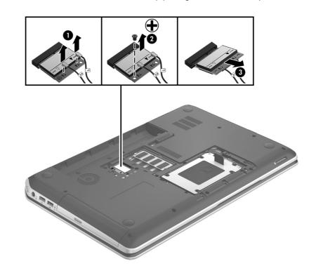
3. Remove the WLAN module (3) by pulling the module away from the slot at an angle.
