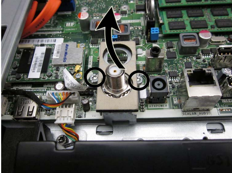
Figure 7-46 Removing the cable connector
