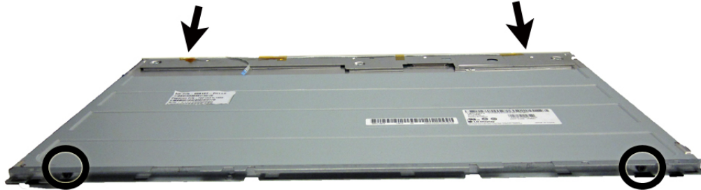
Figure 7-62 Display panel bracket location
