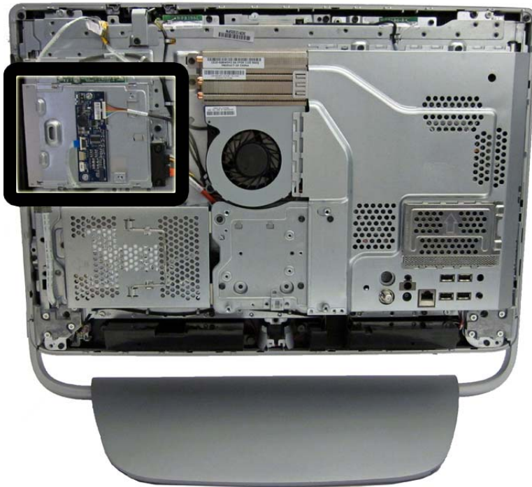
Figure 7-6 Optical drive location
