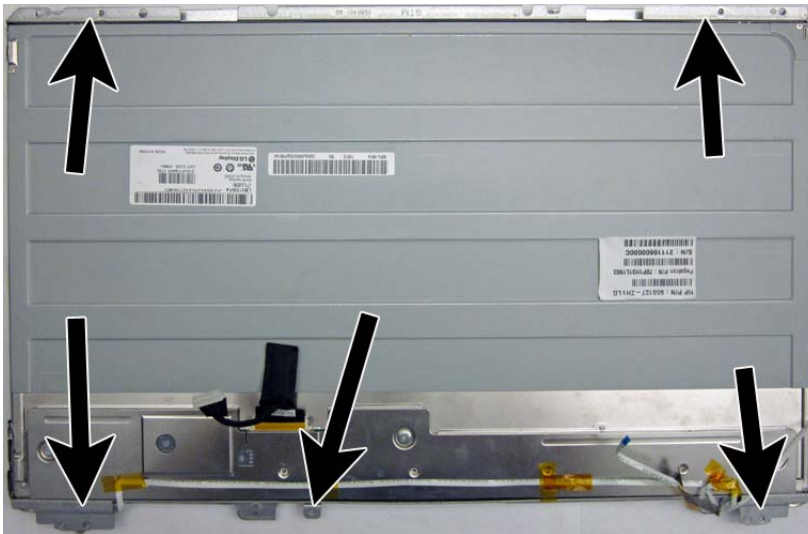
Figure 7-62 Display panel bracket location
