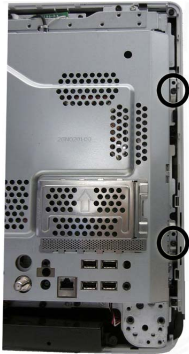
Figure 7-55 Removing the middle frame screws – right
