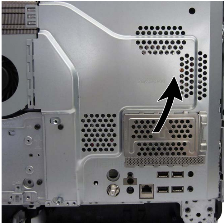
Figure 7-3 Removing the memory cover
