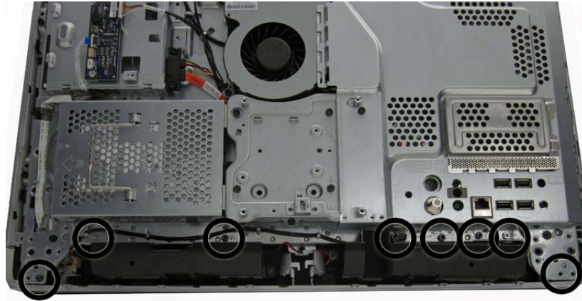
Figure 7-57 Removing the middle frame screws – bottom
