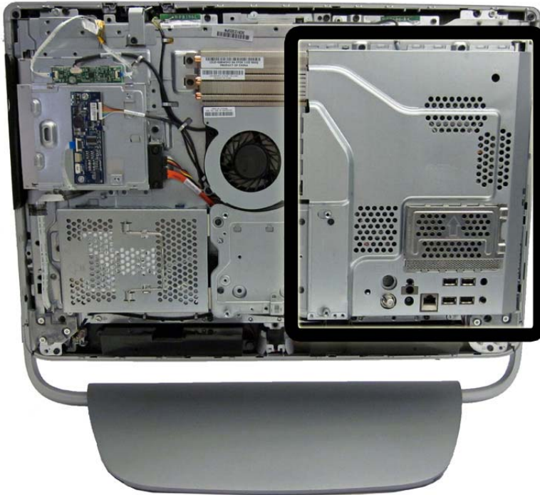
Figure 7-24 System board cover location
