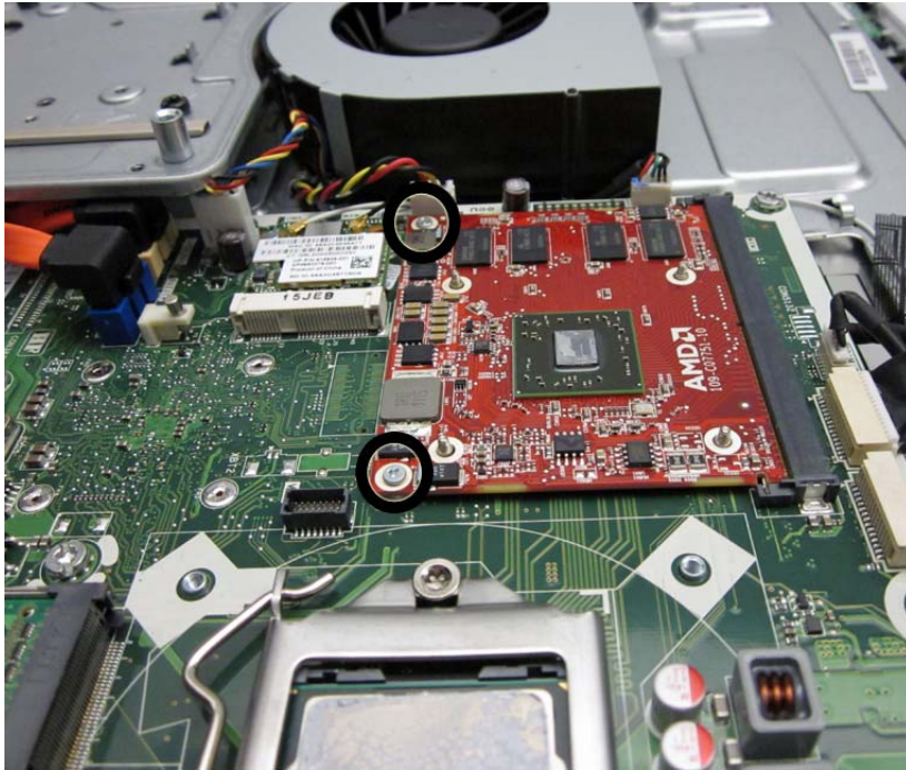
Figure 7-37 Removing the graphics card
