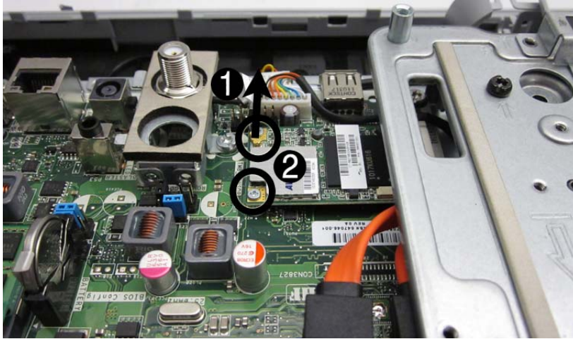
Figure 7-30 Removing the TV tuner module antenna and screws
