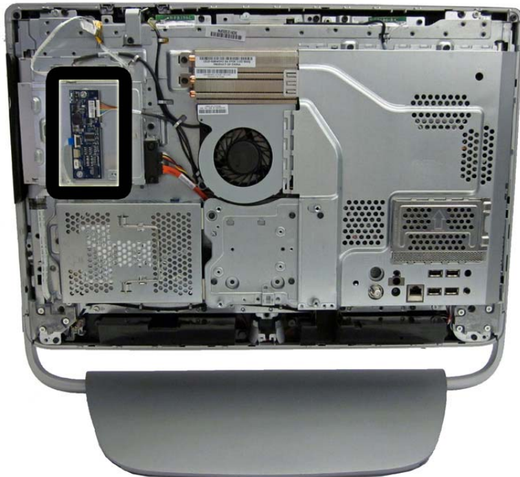
Figure 7-12 converter board location
