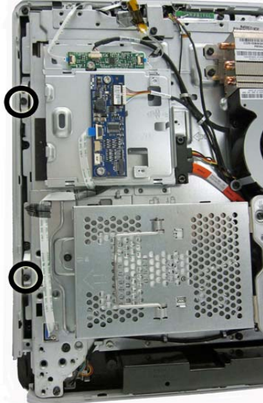
Figure 7-54 Removing the middle frame screws – left
