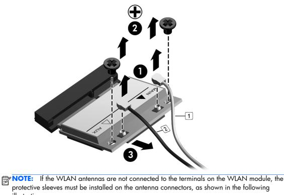
protective sleeves must be installed on the antenna connectors, as shown in the following illustration.
