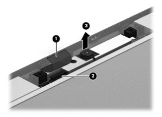
If you need to remove the display panel, remove the 6 Phillips PM1.5×3.0 screws (1) that secure the display panel to the display enclosure, and then rotate the top of the panel up to remove it (2).
