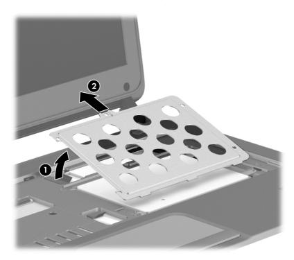
4. Pull the hard drive tab (1) toward the edge of the computer to disconnect the hard drive.
