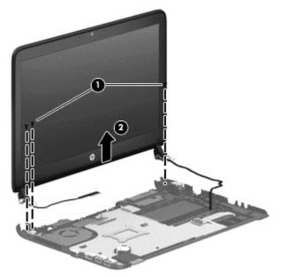
**CAUTION:** When reinstalling the display assembly, be sure that the wireless antenna cables are routed and arranged properly.
