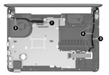
7. Remove the 2 Phillips PM2.0×4.0 screws (1) that secure the power connector bracket to the computer.
