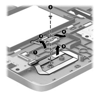
Reverse this procedure to install the fingerprint reader board.
