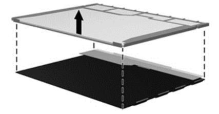
**24.** Recycle the LCD panel and backlight.
