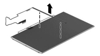
**19.** If it is necessary to replace the display hinges, remove the 6 Phillips PM2.5×3.0 screws **(1)** that secure the display hinges to the display enclosure, and then lift the hinges from the enclosure **(2)**.
