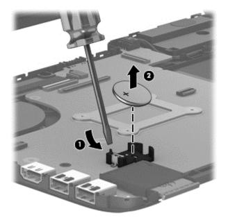
Reverse this procedure to install the RTC battery.
