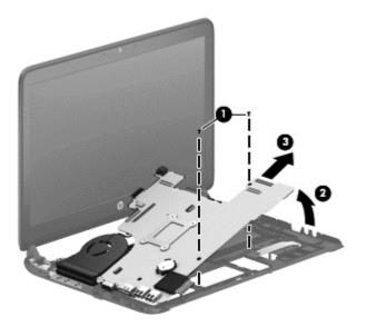
5. If you need to remove the security bracket from the computer, remove the Phillips PM2.0×3.0 screw (1) that secures the brakcet to the base enclosure, and then lift the bracket straight up and off the computer (2).
