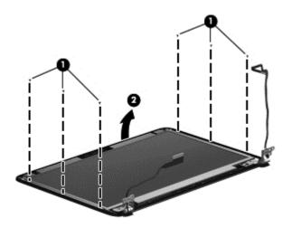
If you need to remove the display panel/webcam cable, disconnect the cable by lifting the tape
