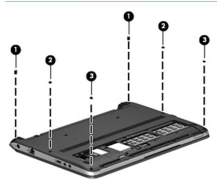
3. Remove the 10 Torx T8M2.5×5.0 screws that secure the top cover to the computer.
