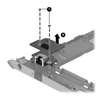
Reverse this procedure to install the function board.
