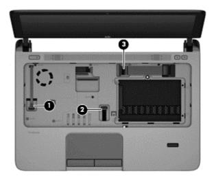
8. Pry up on the top of the top cover (start near the hard drive) to disengage it from the computer, and then remove the top cover from the computer.
