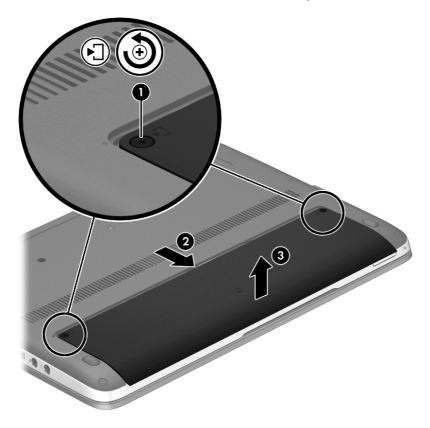
Reverse the removal procedures to install the service door.
