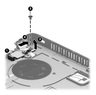
Reverse this procedure to install the power button board.
