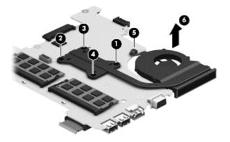
**NOTE:** Thoroughly clean thermal material from the surface of the system board **(1)** and heat sink **(2)** each time you remove the heat sink. All heat sink and processor spare part kits include thermal material.
