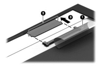
**18.** Remove the display/webcam cable from the back of the display panel.
