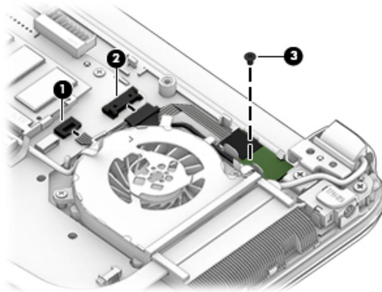
4. Press the tab that secures the board to the computer **(1)**, and then remove the power button board and cable from the computer **(2)**.
