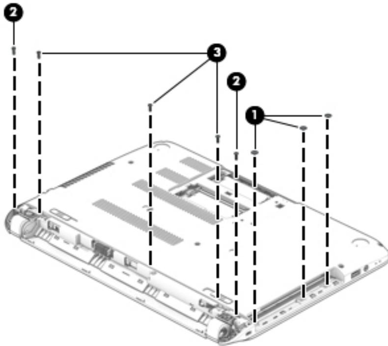
5. Remove the 11 Phillips PM2.5×6.0 screws that secure the bottom cover to the computer.
