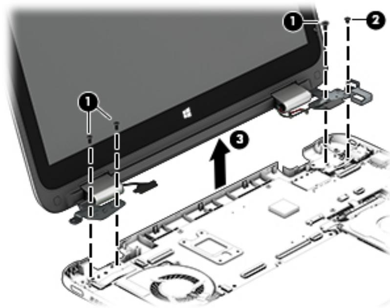
If it is necessary to replace any of the display assembly subcomponents:
