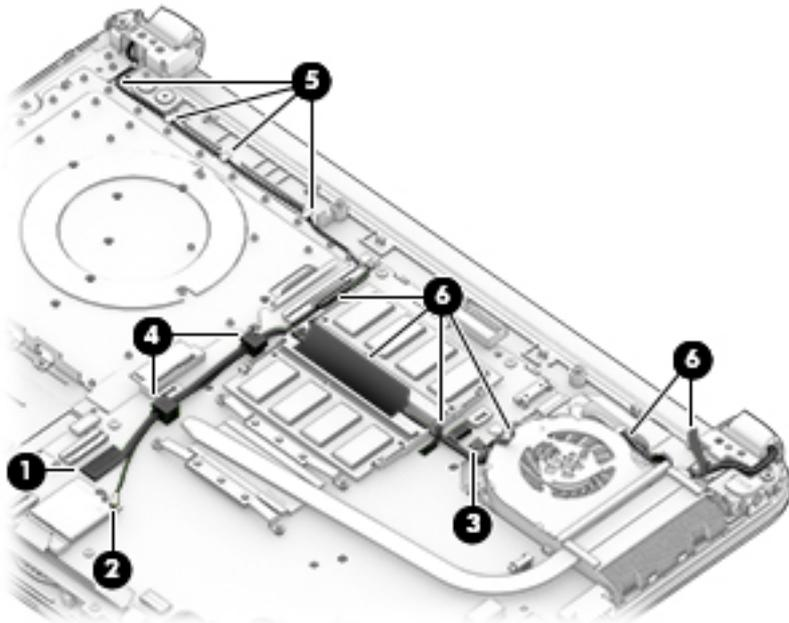
7. Position the computer upright, and then disconnect the following cables from the system board:
