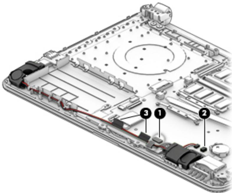
4. Remove the cable from the routing path **(1)**, and then lift up and remove the speakers from the computer **(2)**.
