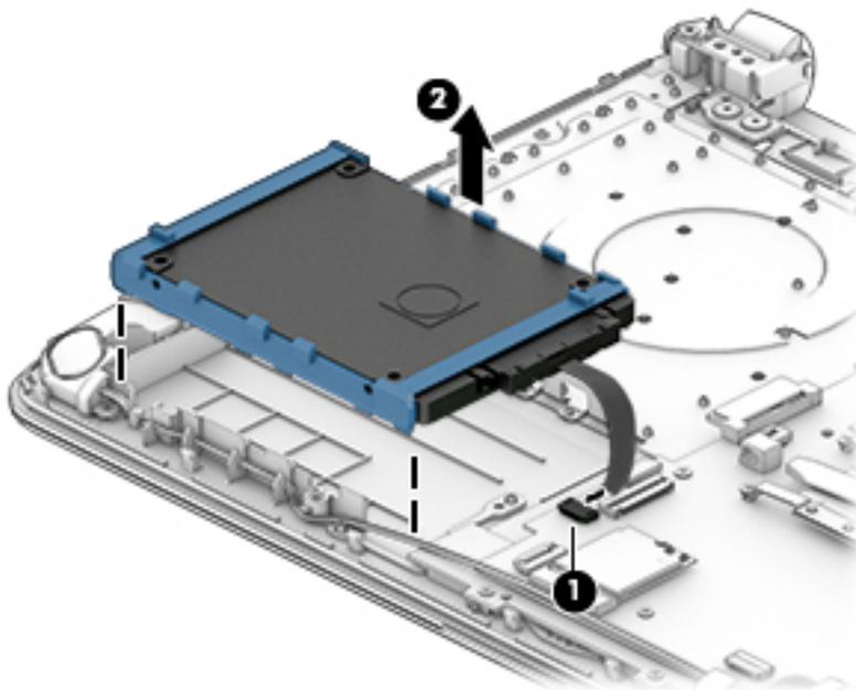
3. To disassemble the hard drive, pull the connector away from the drive to remove it **(1)**.
