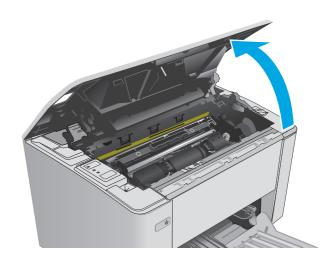
2. Remove the used imaging drum (including the used toner cartridge) from the printer.
