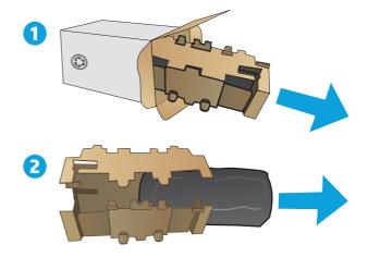
5. Remove the new imaging drum package from the box, and then pull the drum from the protective bag.
