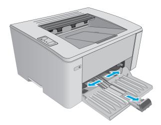
3. Load the paper face-up with the top forward in the input tray.
