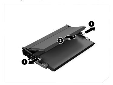
**13.** Slide the new SODIMM **(1)** into the socket at approximately a 30° angle, and then press the SODIMM down **(2)** so that the latches lock it in place.
