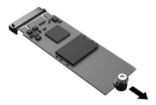
11. Pull the screw kit off of the flash storage module and attach it to the replacement flash storage module.
