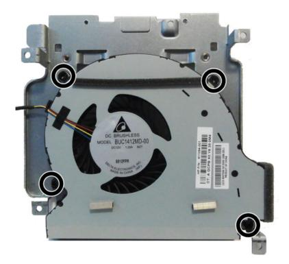
**9.** Separate the fan from the bracket.
