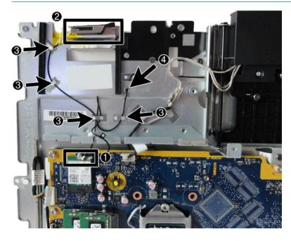
**16.** On the rear of the chassis, note the locations the cables route through **(1)**, and the remove the cables from the clips built into the chassis **(2)**.
