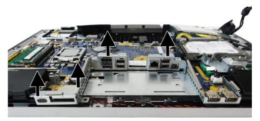
To replace the I/O bracket, reverse the removal procedures.
