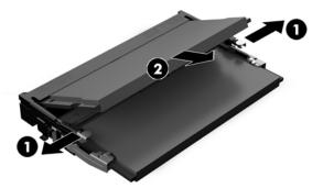
6. Slide the new memory module into the slot at approximately a 30° angle (1), then press the memory module down (2) so that the latches lock it in place.
