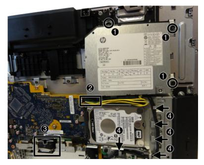
**10.** Remove the power supply from the computer.
