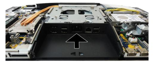
To install the bottom I/O cover, reverse the removal procedures.
