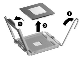
NOTE: After installing a new processor onto the system board, always update the system ROM to ensure that the latest version of the BIOS is being used on the computer. The latest system BIOS can be found on the Web at: <a href="http://www.hp.com">http://www.hp.com</a>.
