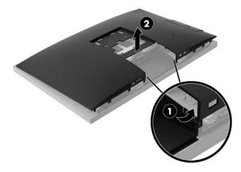
To replace the access panel, reverse the removal procedures.
