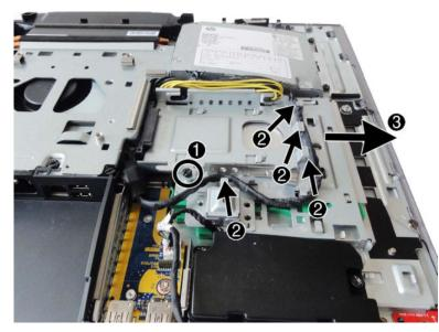
To replace the hard drive cage, reverse the removal procedures.
