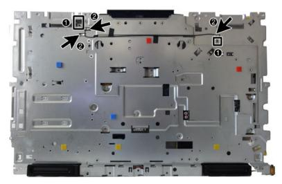
17. Peel the left antenna from the chassis (1), and then pull the other end of the cable through the hole in the chassis (2). Remove the left antenna and cable.
