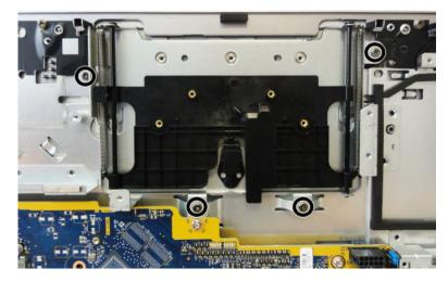
**13.** Remove the webcam bracket from the computer.
