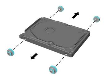
To install a hard drive, reverse the disassembly instructions.
