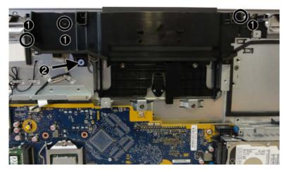
7. Remove the webcam shield from the computer.
