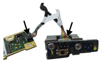
8. If necessary, remove the two Phillips screws that secure the power button board to the bracket.
