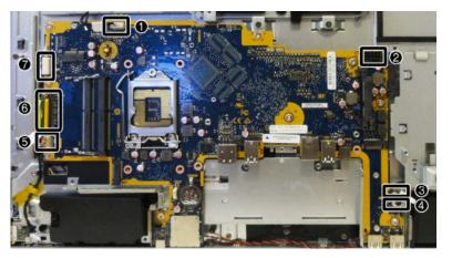
**15.** In the order printed on the system board, remove the nine Torx screws **(1)-(9)** that secure the system board to the computer.
