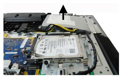
To install the power supply, reverse the removal procedures.
