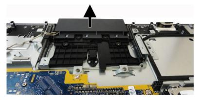
12. If you need to remove the webcam bracket, remove the VESA bracket/fan assembly (<u>VESA mounting</u> <u>bracket/fan assembly on page 43</u>), and then remove the four Torx screws that secure the webcam bracket to the computer.
