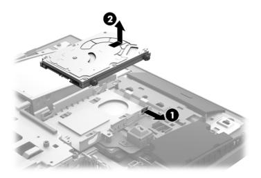
7. Remove the four mounting screws from the 2.5 inch hard drive. Be sure to keep the screws together with the blue rubber grommets to use to install a replacement drive.
