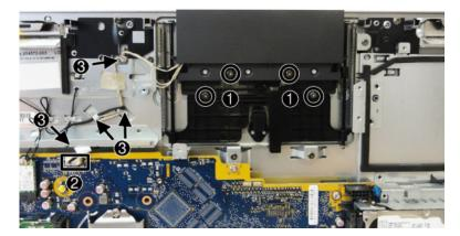
**11.** Remove the webcam assembly from the computer.
