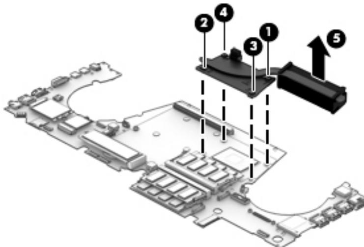
2. The following illustration shows the replacement thermal material locations. The thermal material must be thoroughly cleaned from the surfaces of the heat sink and the system board components each time the heat sink is removed. Replacement thermal material is included with the heat sink and system board spare part kits.
