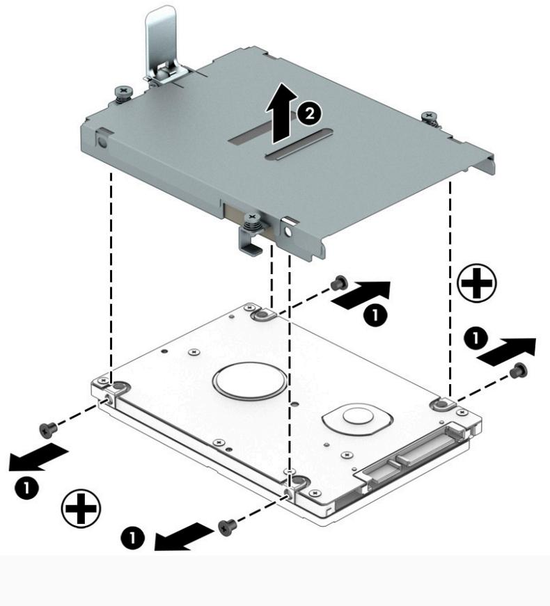
4. **Secondary hard drive:** Remove the bottom cover (see [Service door on page 36](#)).
