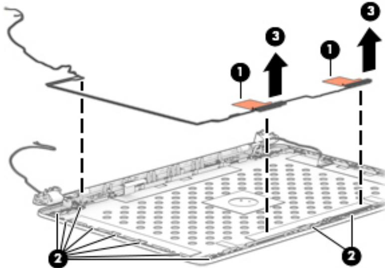
**11.** If it is necessary to replace the display cable:
