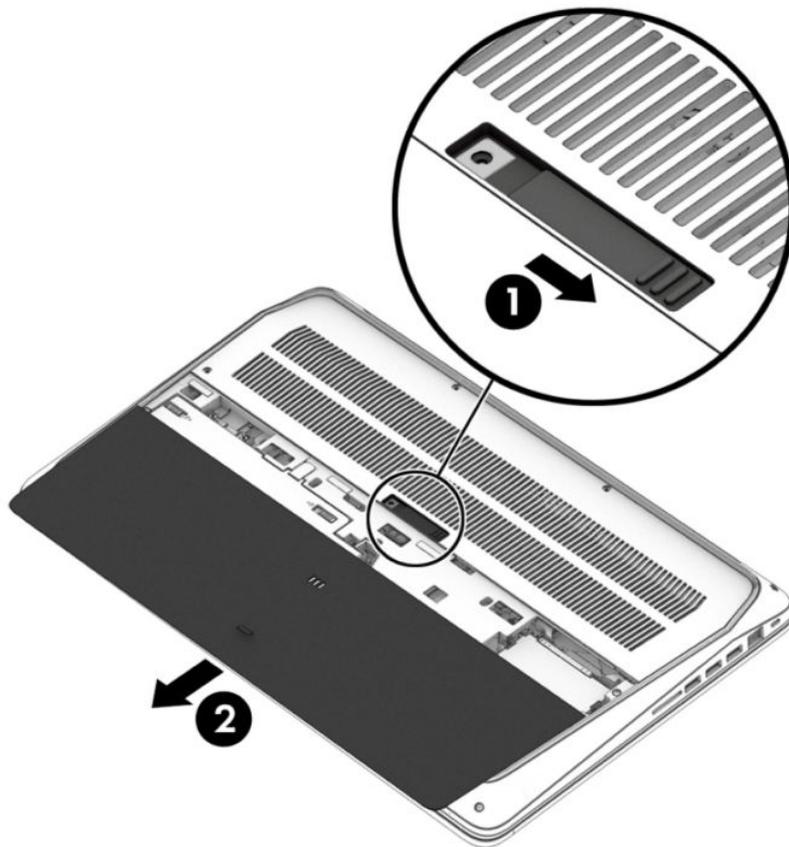
4. Loosen the 14 Torx captive screws **(1)** to release the rear cover.
