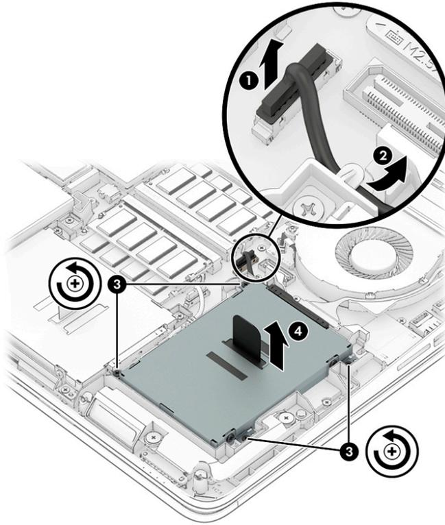
4. Repeat steps 1 through 4 to remove the secondary hard drive.
