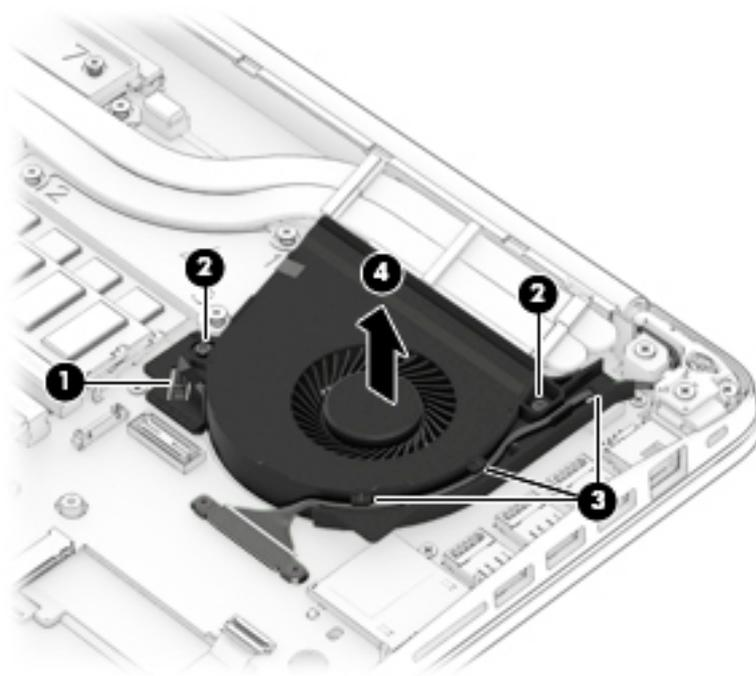
3. Release the fan connection **(1)** on the GPU fan, and then release the two captive screws **(2)** securing the GPU fan to the computer.
