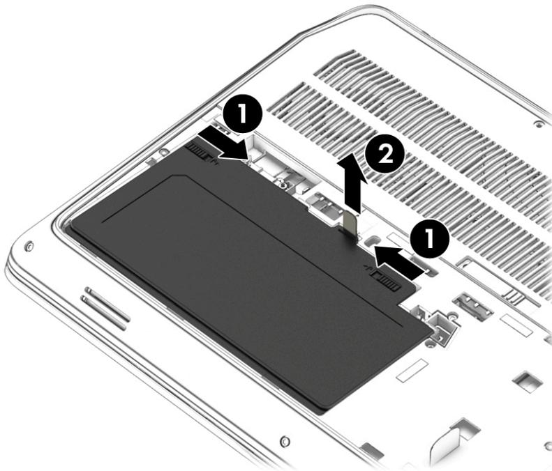
Reverse this procedure to install the battery.
