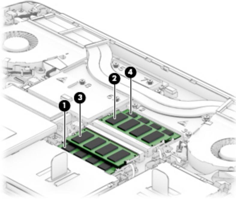
2. Spread the retaining tabs **(1)** on each side of the memory module slot to release the memory module. (The memory module tilts up.)
