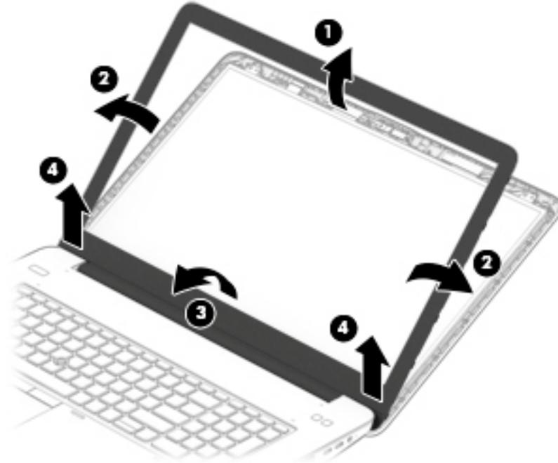
5. If it is necessary to replace the display panel:
