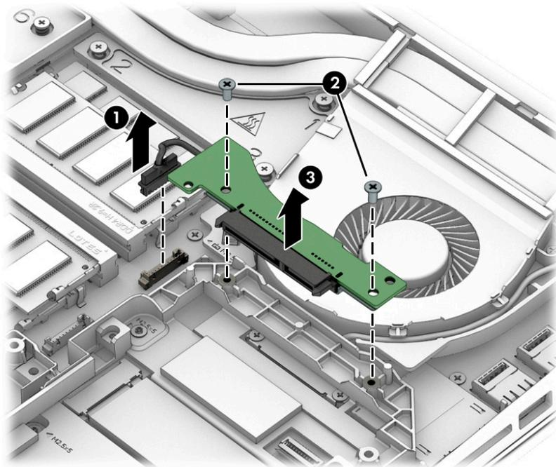
2. If it is necessary to replace the hard drive connector board cable, after removing the board, disconnect the cable from the board.
