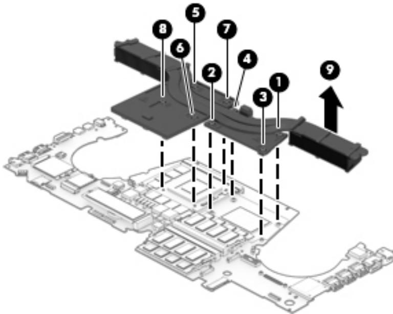
2. The following illustration shows the replacement thermal material locations. The thermal material must be thoroughly cleaned from the surfaces of the heat sink and the system board components each time the heat sink is removed. Replacement thermal material is included with the heat sink and system board spare part kits.
