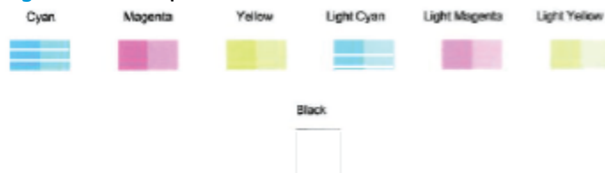
Figure 8-2 Example of color blocks with defects
