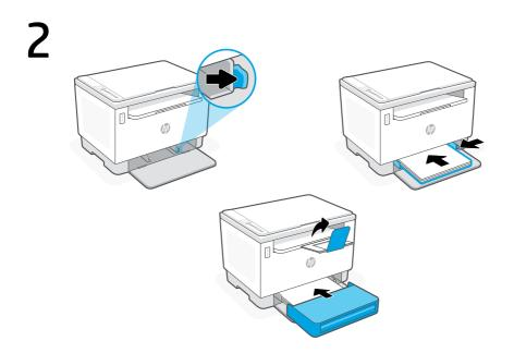
Adjust guides, load paper and slide the tray cover into place. Open the output tray extender.
