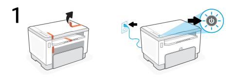
Remove all packaging and tape. Plug in and power on the printer.
